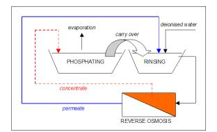
Figure 2. Principle flow diagram closed loop phosphating with reverse osmosis
