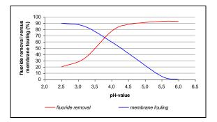
Figure 4. Influence of pH-value on fluoride removal and membrane fouling
