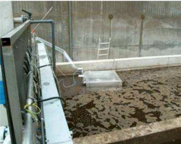
Picture 2. Lindvall box at the surface of a denitrification tank
