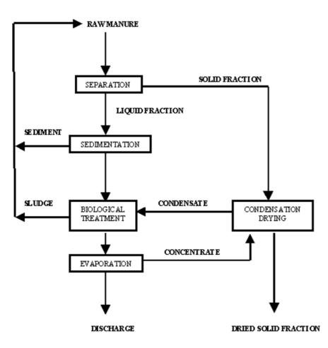
Figure 1. Flowchart of the Trevi manure treatment concept
