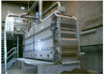
Picture 3. Condensation drier with drying unit in front and heat-exchanging unit on top
